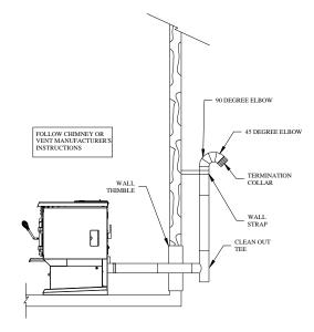
Figure 7 Venting through wall
